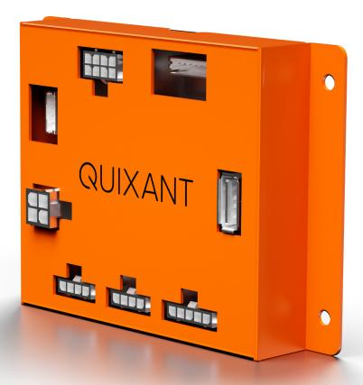
Its flexible design makes it an innovative solution to create eye-catching cabinet LED lighting effects on, which can be synchronised with in-game graphics. It can operate as a standalone LED controller or can be managed through a USB interface using Illuminate, Quixant's Cabinet LED software solution, which is embedded on Quixant's range of platforms as standard.
